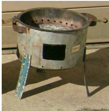
Figure 4: Mirak stove: height: 32 cm; diameter: 30.5 cm; and weight: 2.8 kg.
