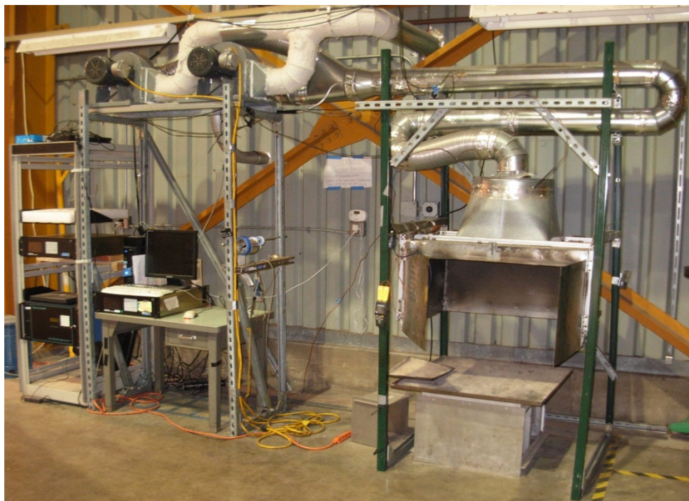
Figure 2: The stove testing system at LBNL. The exhaust hood and ductwork is on the right-hand side of the photo, while the instrumentation is on the left.
