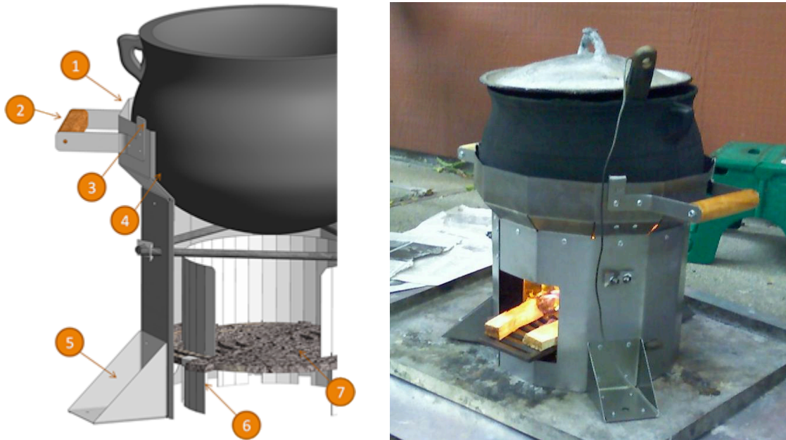
Figure 2: Schematic and picture of the Berkeley-Darfur Stove. The schematic illustrates several design features that are described in the text above.
